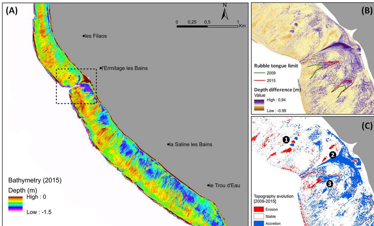
Fig. 7. Digital elevation model extracted from the 2015 hyperspectral image (A), differential bathymetry and the delineation of rubble tongues RT01 and RT02 (B) and topographic change estimated between 2009 and 2015 (C) in the Ermitage Pass area (dashed box). Numbers indicate the main identified geomorphologic features.
